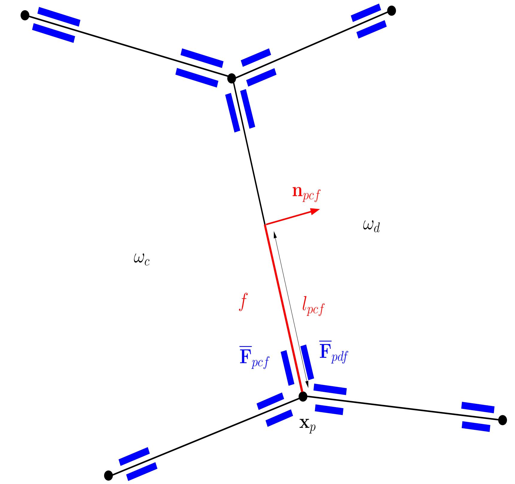
The multi-dimensional numerical flux corresponds to the classical one-dimensional numerical flux + nodal contribution from the node velocity  $\mathbf{v}_p$
