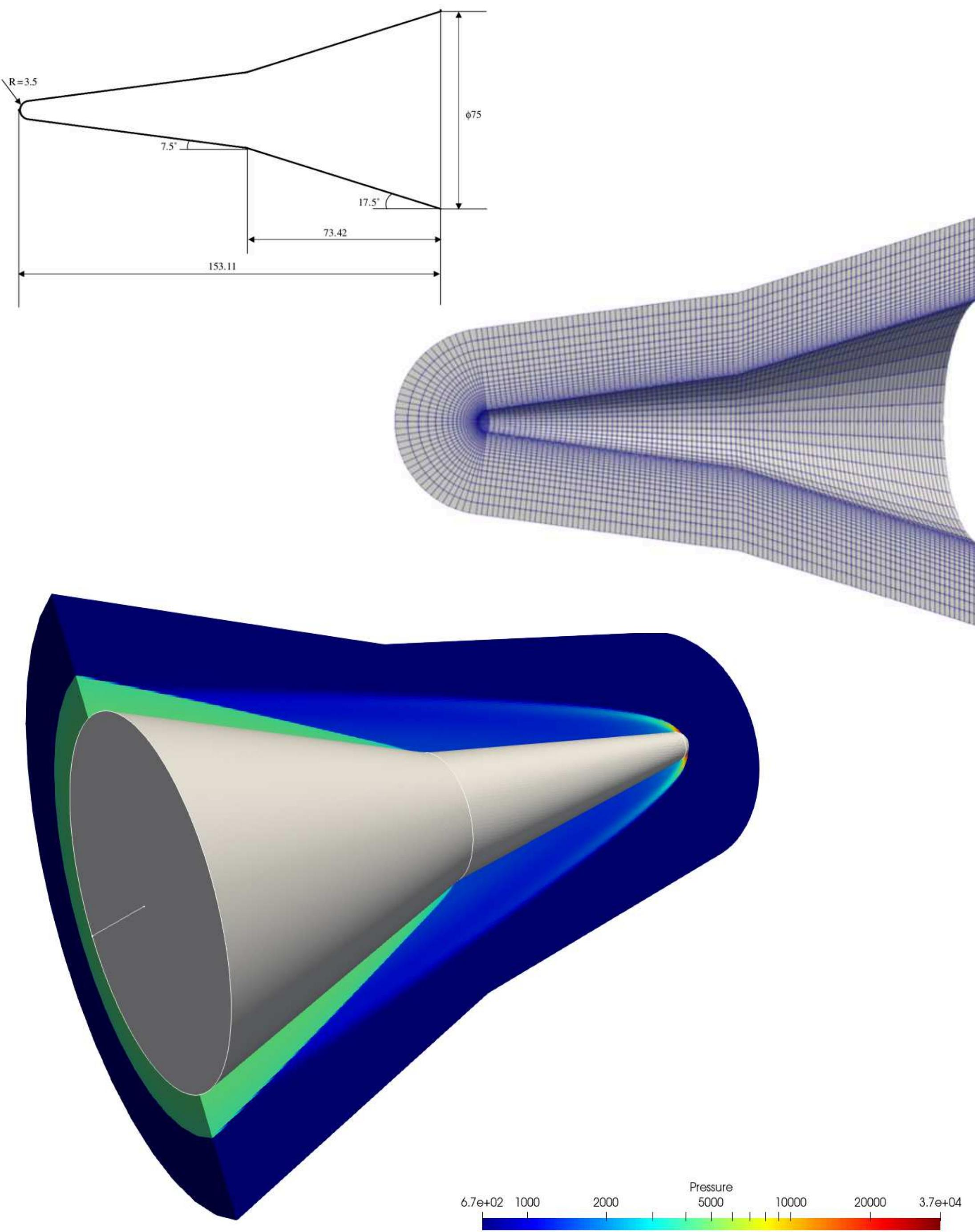
Comparison of our 3D solver and a structured 2D axisymmetric solver<sup>[16]</sup>.
