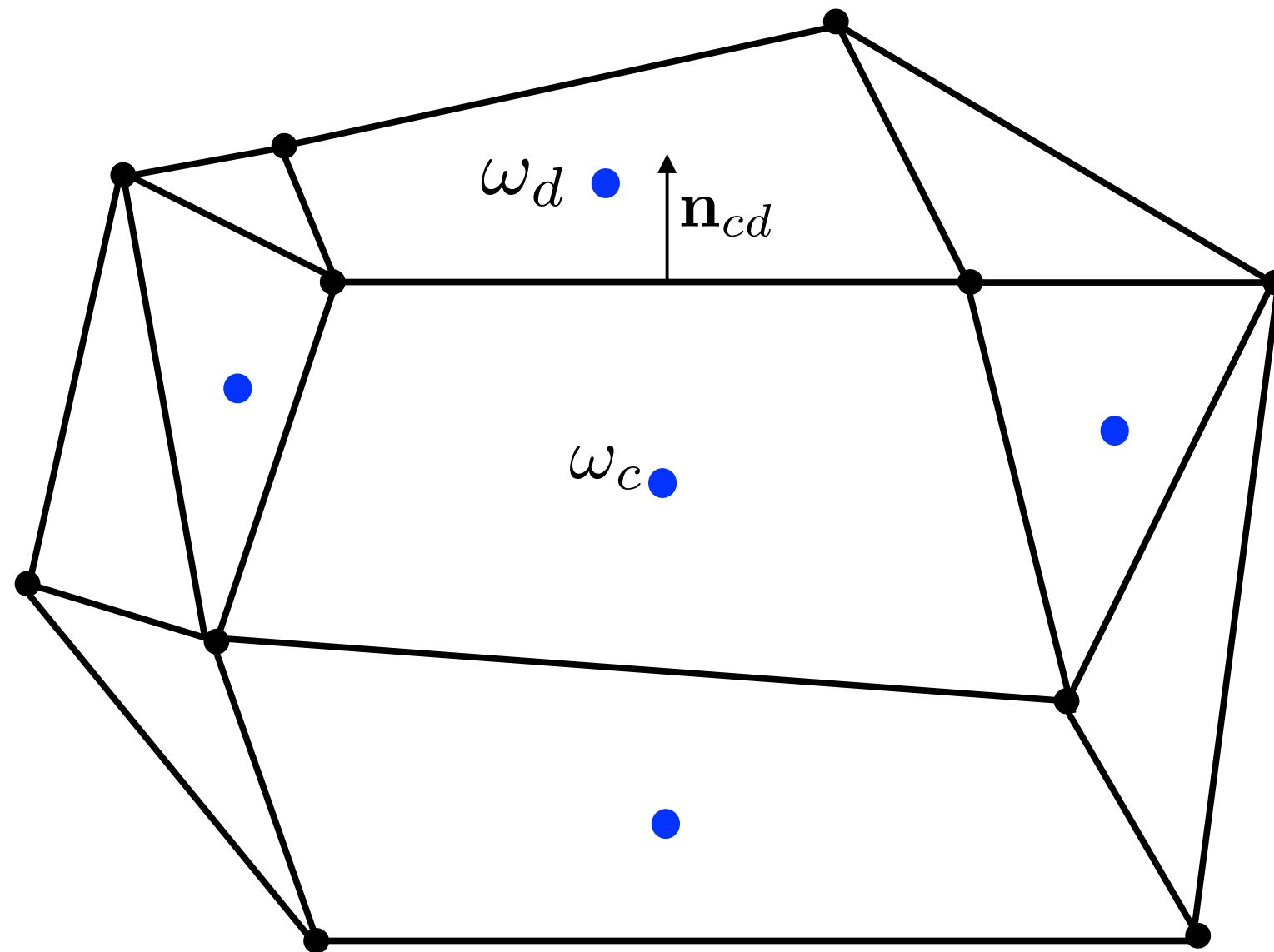
Subsurface-based FV scheme - Multi-point scheme
