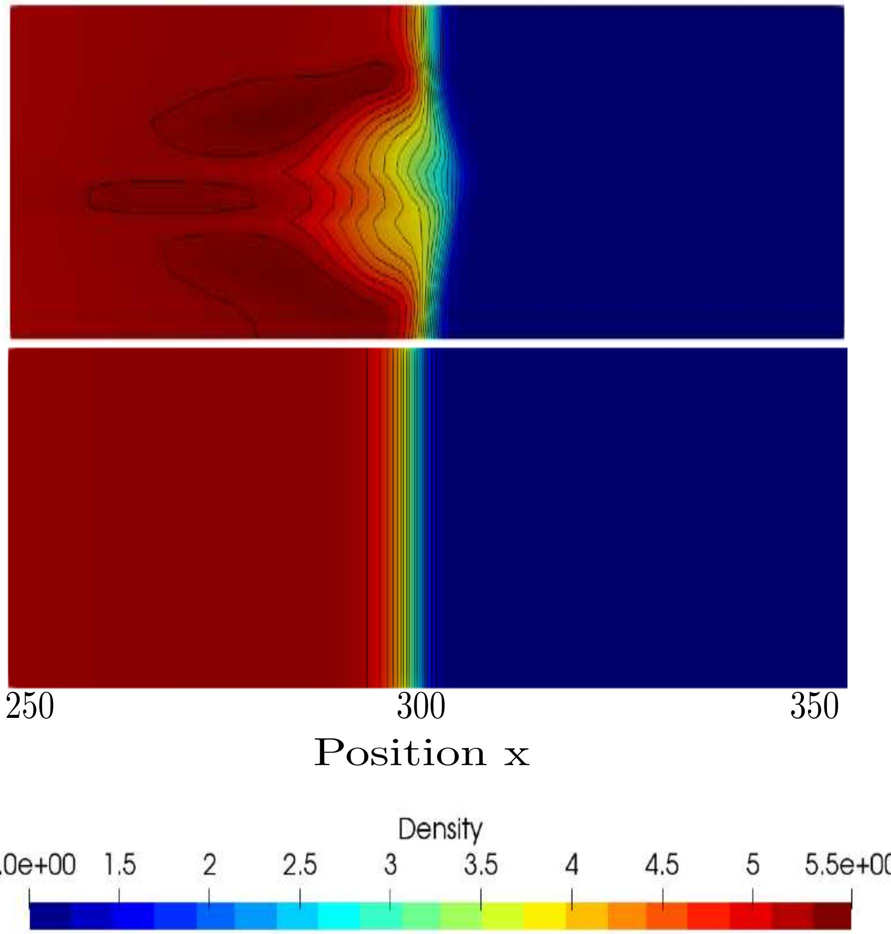
Comparison of first-order two-point solver and multi-point solver.
