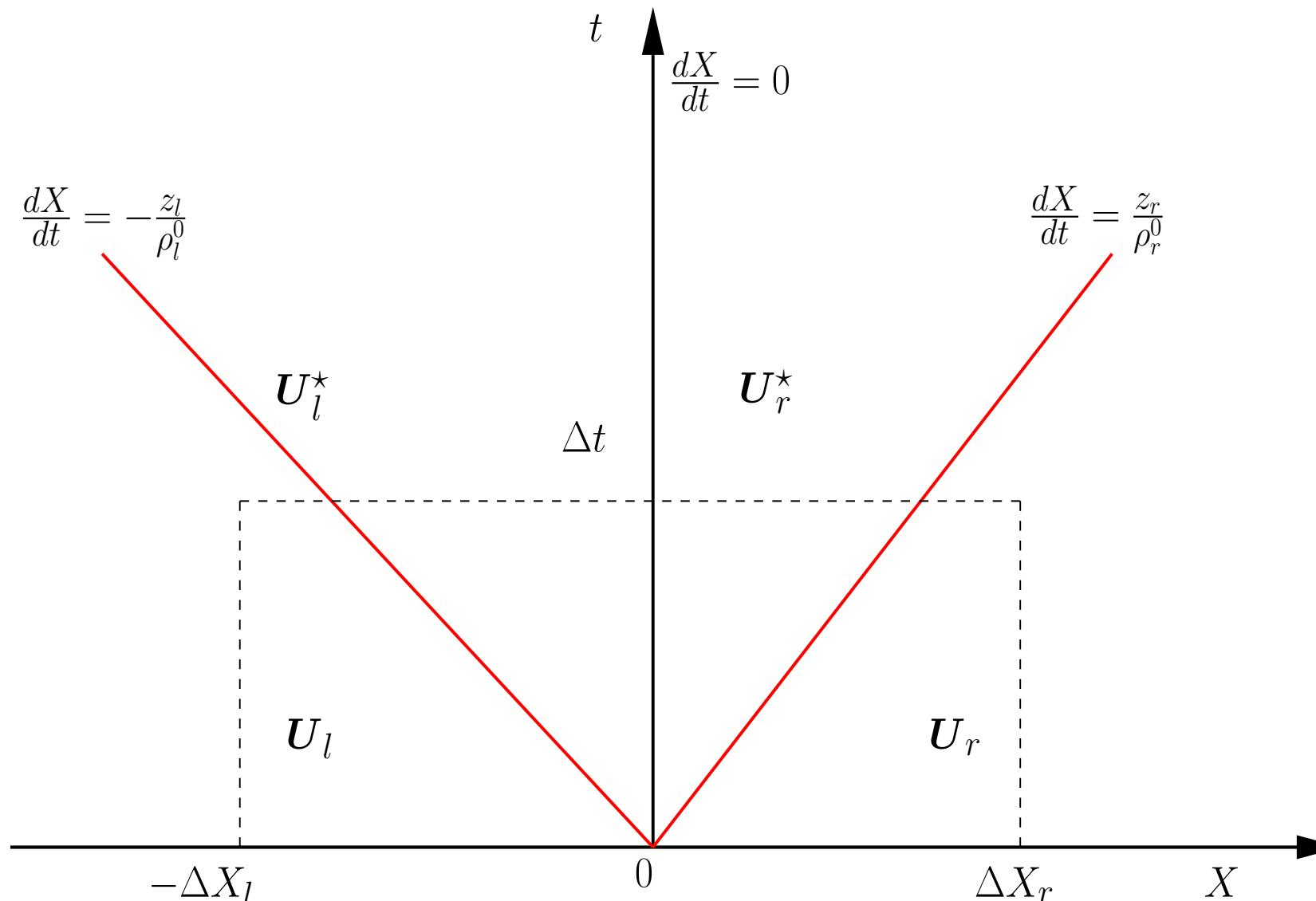
$$\frac{\partial \mathbf{V}}{\partial t} + \frac{\partial \mathbf{G}}{\partial m} = \mathbf{0}, \quad \mathbf{V}(x,0) = \begin{cases} \mathbf{V}_l & \text{if } m < 0, \\ \mathbf{V}_r & \text{if } m \geq 0, \end{cases}$$
